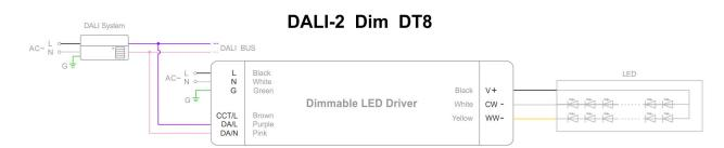
DALI-2 dimming with intelligent device, DALI master and dimmer
